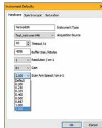
Quick scanning with FTIR allows for very quick response times with measurement update times of the order 0.2sec (5Hz)
