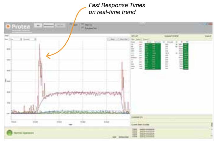
Quick scanning with FTIR allows for very quick response times with measurement update times of the order 0.2sec (5Hz)
