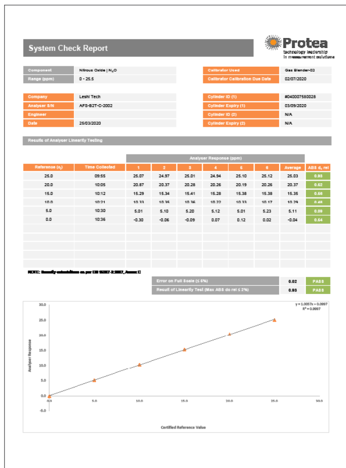
Calibration workbook provided with atmosCAL gives EN and ISO calculations for the user
