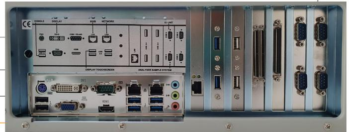
**Figure 3:** Wide range of connectivity and communications as standard - 3x Ethernet, 6x Serial, 12x USB, 64-ch AIO, 128-ch DIO as standard
