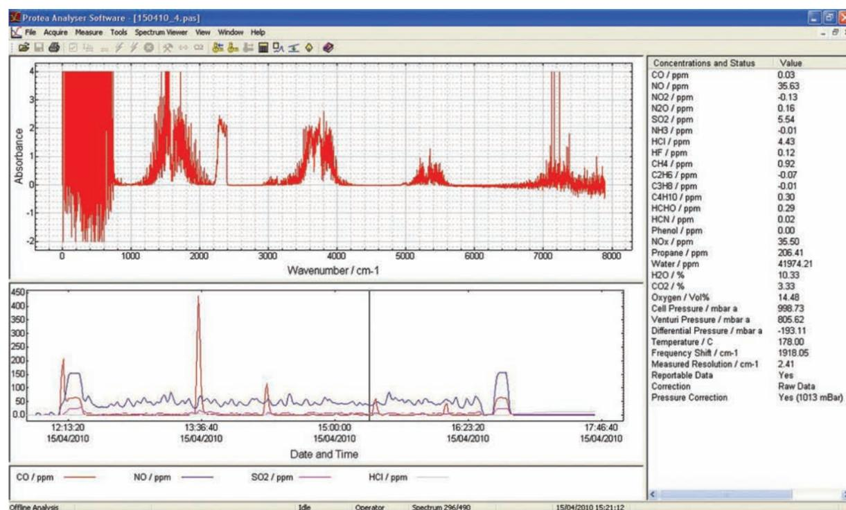
Figure 1: Powerful FTIR Spectral Analysis Software
