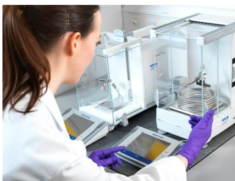
Figure 3: Reference mixtures are prepared by weighing each component
